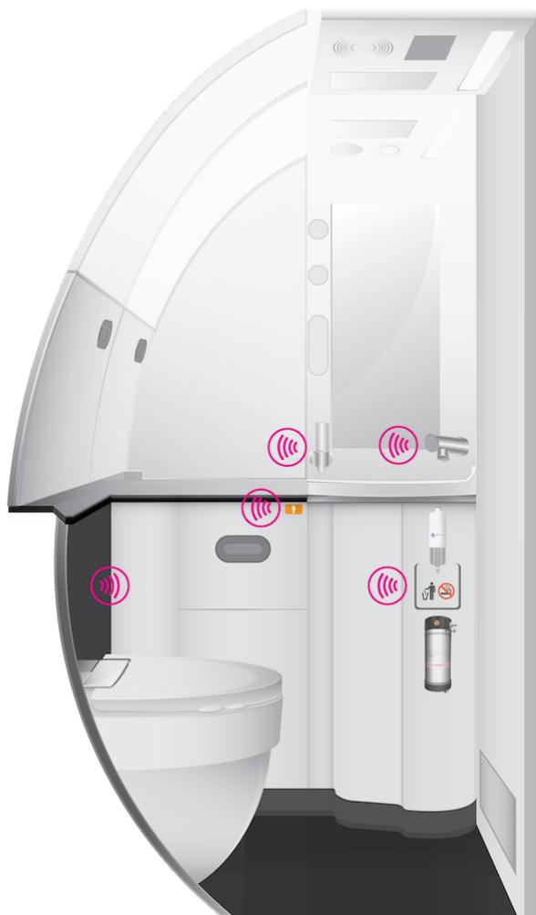
The Healthy Lav by International Water-Guard includes touchless faucet, touchless flush, the 'HE' (high efficiency) lavatory water heater and the UVL1 LED water disinfection unit
