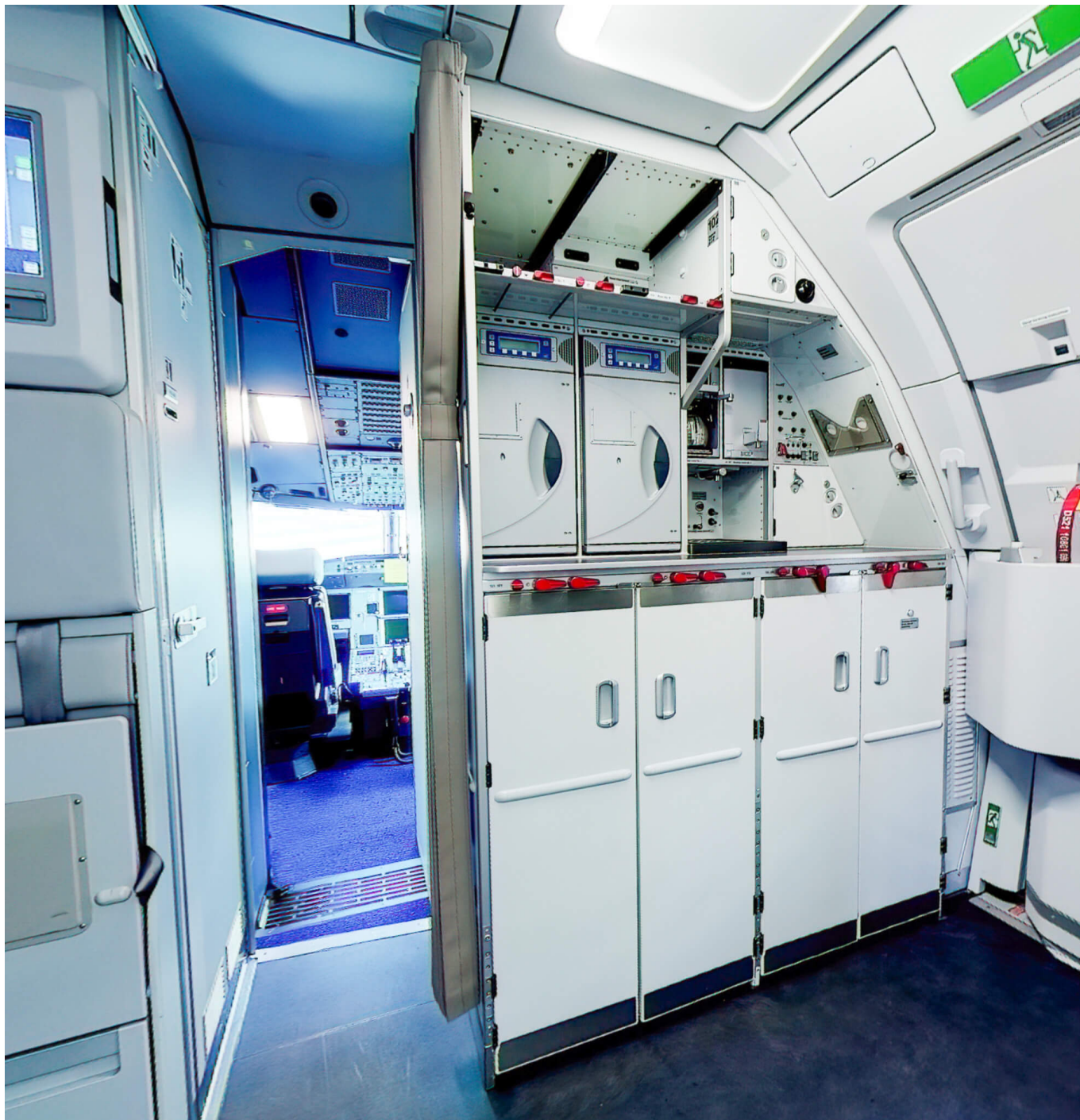
A Bucher single-aisle forward galley
