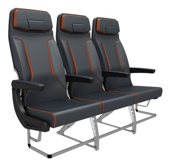
The Elemento by Geven is designed to provide more living space in reduced confines of pitch and has a video screen, cup holder, eyeglass holder, literature pockets, personal electronic device holders and reading lights
