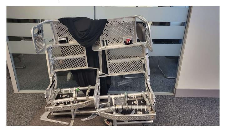
The still intact seat underwent a successful dynamic test, including pitch and roll
