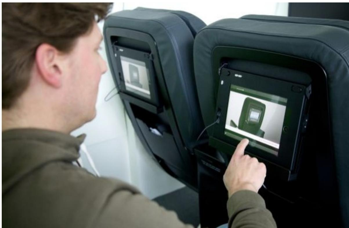
Lufthansa Technik and Qantas Airways have developed a new IFE concept that makes it possible to use a tablet via the seatback throughout the entire flight, rather than a fixed monitor.
