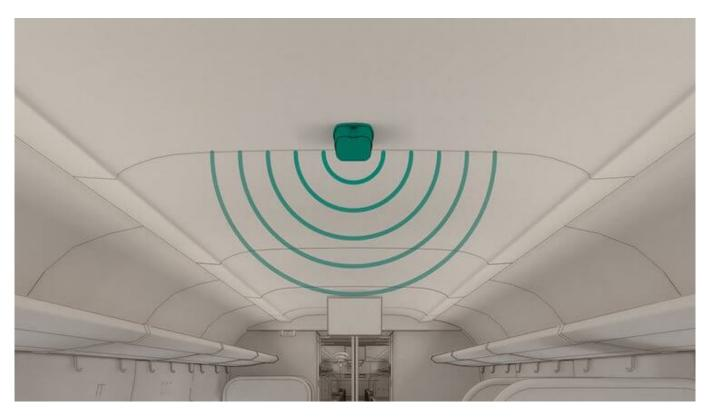
SENCITY Rail ACTIVE In-Carriage antenna can provide multiple access points along the carriage ceiling
