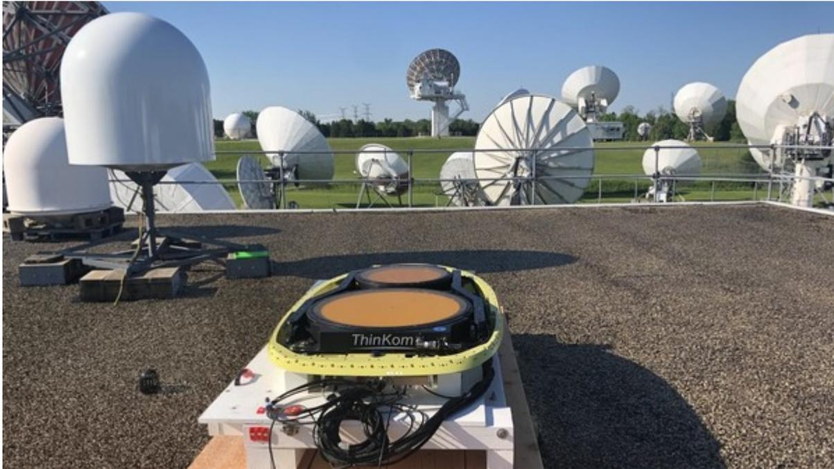
ThinKom Ka2417 phased-array antenna undergoes live tests on Telesat LEO satellite.
